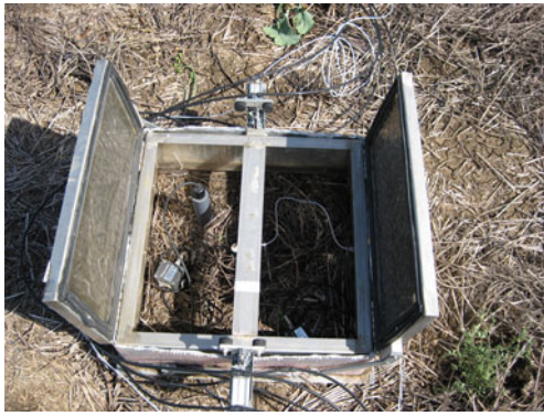
Fig. 4 Chamber used to quantify \text{N}_2\text{O} emissions from legume residues. The lid of a chamber in one of the four replicates of each treatment automatically closes on a rotational basis each hour of the day to continually monitor changes in concentrations of \text{N}_2\text{O} in the chamber headspace. Photo: M. B. Peoples, CSIRO
