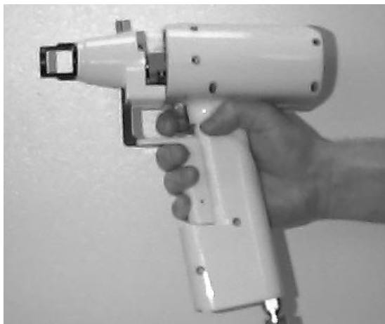
Fig. 16. Position of hand over the safety interlock switch in preparation for firing.
