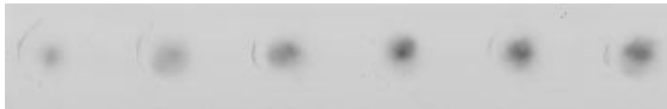
Fig. 25. Representative bombardment showing penetration of 1.6 \mu gold particles into Parafilm at (left to right) 100, 200, 300, 400, 500, and 600 psi using the Helios Gene Gun.
